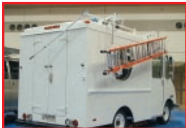
Model 282 EZ-GLIDE™ System Rack mounted on a 10' high cube van with rear slide down system.
