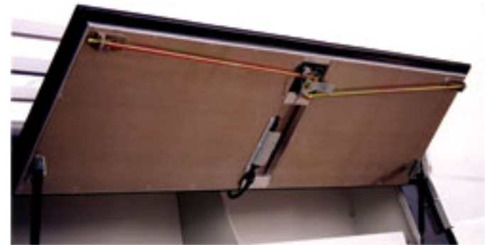
Inside Door Skin Reduces Dents From Shifting Cargo
